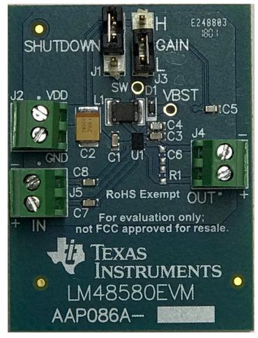
Figure 1. LM48580 Demonstration Board
