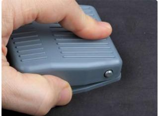
Press down on the top half of the switch to align the holes and insert the hinge pin. Make sure that the notch in the hinge pin is positioned to line up with the small locking pin you removed earlier.
