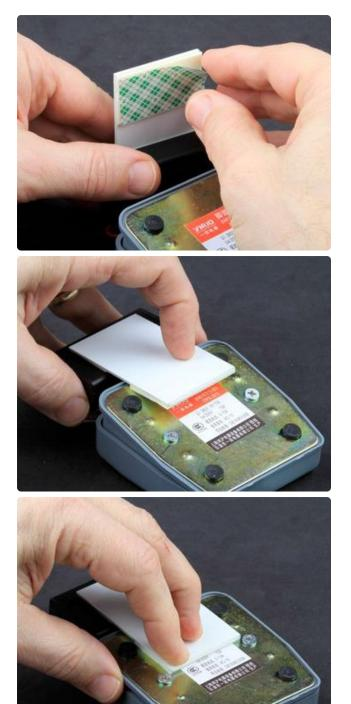
Position the plastic plate over the bottom of the switch and press firmly.
