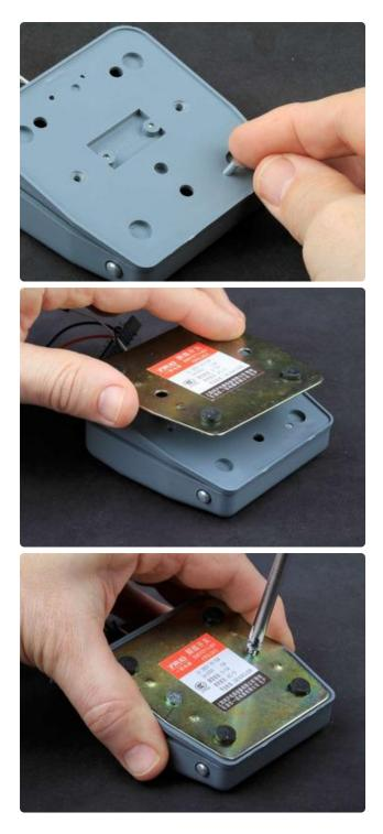
Re-install the locking pin and replace the bottom cover.
