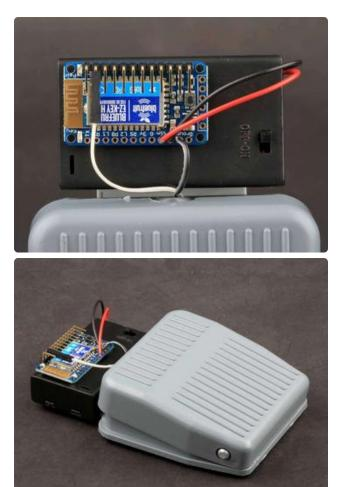
Connect the jumper to pin #1 of the rightangle header. And you are ready to go!
