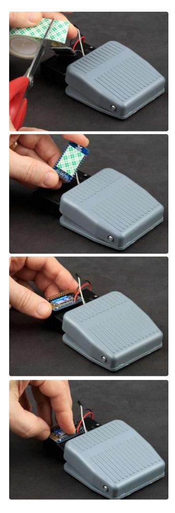
Cut another piece of tape to fit on the bottom side of the EZ-Key. Mount the EZ-Key to the top of the battery box. Keep to the left so you don't cover the ON/OFF switch.
