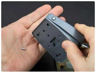
Locate and remove the small locking-pin near the front edge of the switch. It should fall out easily when you turn it over.
