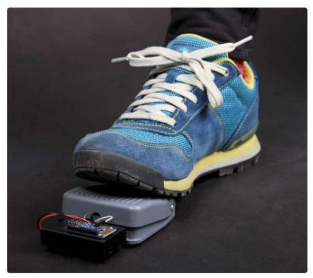
This is a quick and easy project that will be speed your work on future projects. By combining an Adafruit BlueFruit EZ-Key with a foot switch, we end up with a wireless, hands-free scroll button. No need to put down that hot iron to see the next step in the tutorial. Just give the pedal a tap with your foot to scroll down the page.
