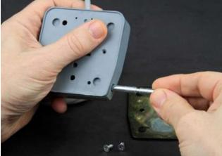
Push on the end of the hinge-pin with the tip of the screwdriver. While squeezing the foot switch, pull the hinge pin completely out.
