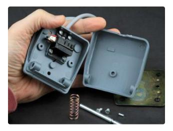
Carefully open the switch and remove the spring.
