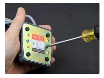
Remove the two screws from the bottom of the foot switch. Remove the bottom plate being careful to keep the bottom of the switch facing up.
