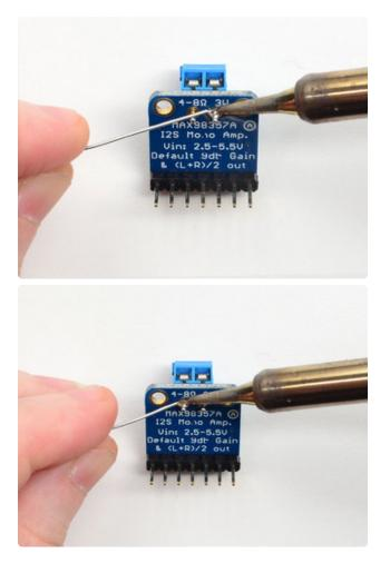
Solder in both pins with plenty of solder!
