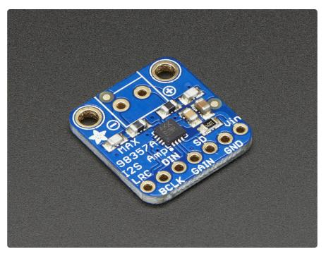
If your microcontroller or microcomputer has digital audio capability, this amp is for you! It takes standard I2S digital audio input and, not only decodes it into analog, but also amplifies it directly into a speaker. Perfect for adding compact amplified sound, it takes 2 breakouts (I2S DAC + Amp) and combines them into one.
