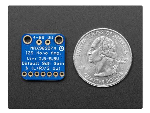
There's a Gain pin that can be manipulated to change the gain. By default, the amp will give you **9dB** of gain. By connecting a pullup or pull down resistor, or wiring directly, the Gain pin can be set up to give 3dB, 6dB, 9dB, 12dB or 15dB.
