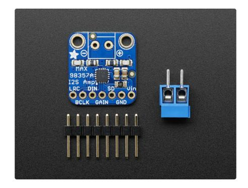
Comes as an assembled and tested breakout board, with a small piece of optional header and 3.5mm terminal block. Some soldering is required to attach the header and terminal block if those are desired.
