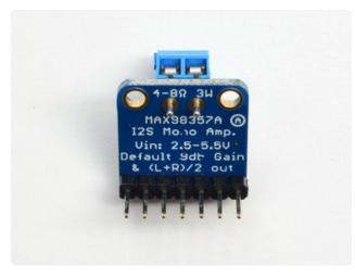
If you want to use a terminal block for connecting a speaker, place the 3.5mm terminal so the mouthes point out.
