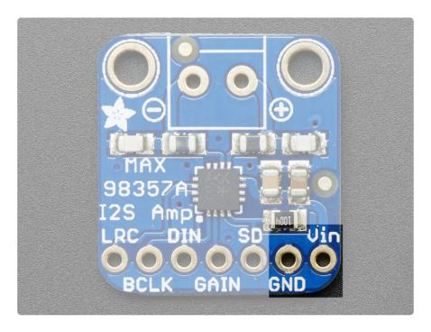
This is the power for the amplifier and logic of the amplifier. You can provide 2.5V up to 5.5V. Note that at 5V you can end up putting up to 2.8W into your speaker, so make sure your power supply can easily handle up to 650mA and we recommend a power supply spec'd for at least 800mA to give yourself some 'room'
