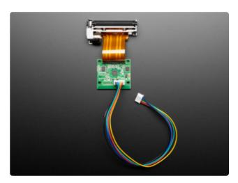
For the most peculiar situations not covered above, the **Thermal Printer Receipt Guts** (http://adafru.it/2753) is just the insides of a thermal printer. You will need to design and build an enclosure to mount the hardware and hold a paper roll...in principle, any length roll can then work with this.
