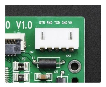
The pin order here is **not the same** as the Tiny or Nano printers. And if you have both Guts and Nano printers, be super careful about the wiring, because the plugs are interchangeable but the sequence of wires and colors (if any) do not have the same functions!
