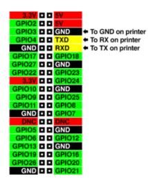
Now the printer can be connected without making a mess.
