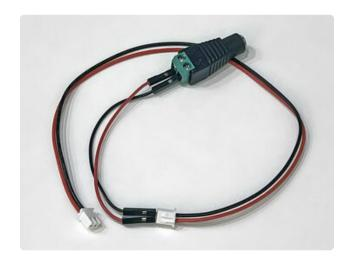
During initial testing and for quick temporary projects, it's usually okay to jam breadboard prototyping wires (http://adafru.it/1956) into the end connector on the DC power cable (or power+serial cable on Nano and guts), and the other end to a DC barrel jack adapter.
