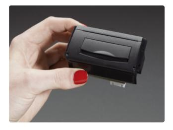
For the most compact and portable situations, the Nano Thermal Receipt Printer (http://adafru.it/2752) is smaller still, accommodating a 5m/16' paper roll (http://adafru.it/2755).
