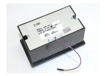
Screw the controller board back in place (check that neither of the cables has come unseated), routing the DTR wire around between the two sockets, then screw the back on.
